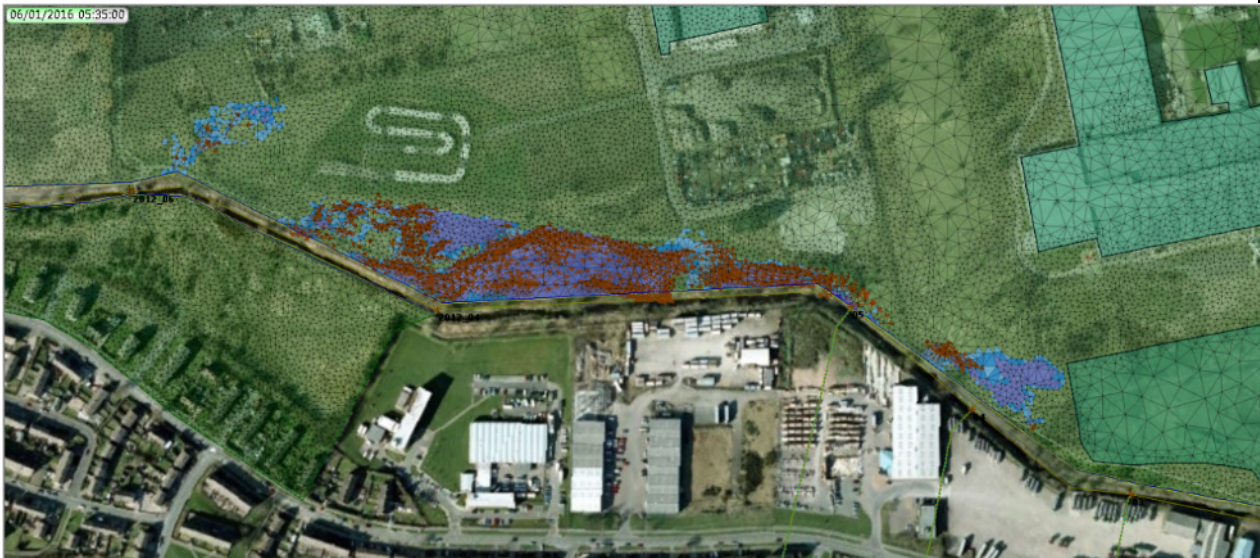
Figure 5c: Water travelling from node 2012_06 northwards and moving eastwards towards the back of the BMX track and spill downstream of node 05.
