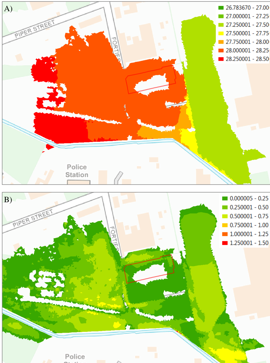
Figure 11. Maximum water levels (A) and depths (B) in the study area for the 1 in 200yr event under existing conditions. Development footprint is marked by the red polygon. The absence of flooded area to the west of the site in A) is due to the legend setting, which has a maximum of 28.5mAOD for clarity. Flooding occurs, as seen in B).
