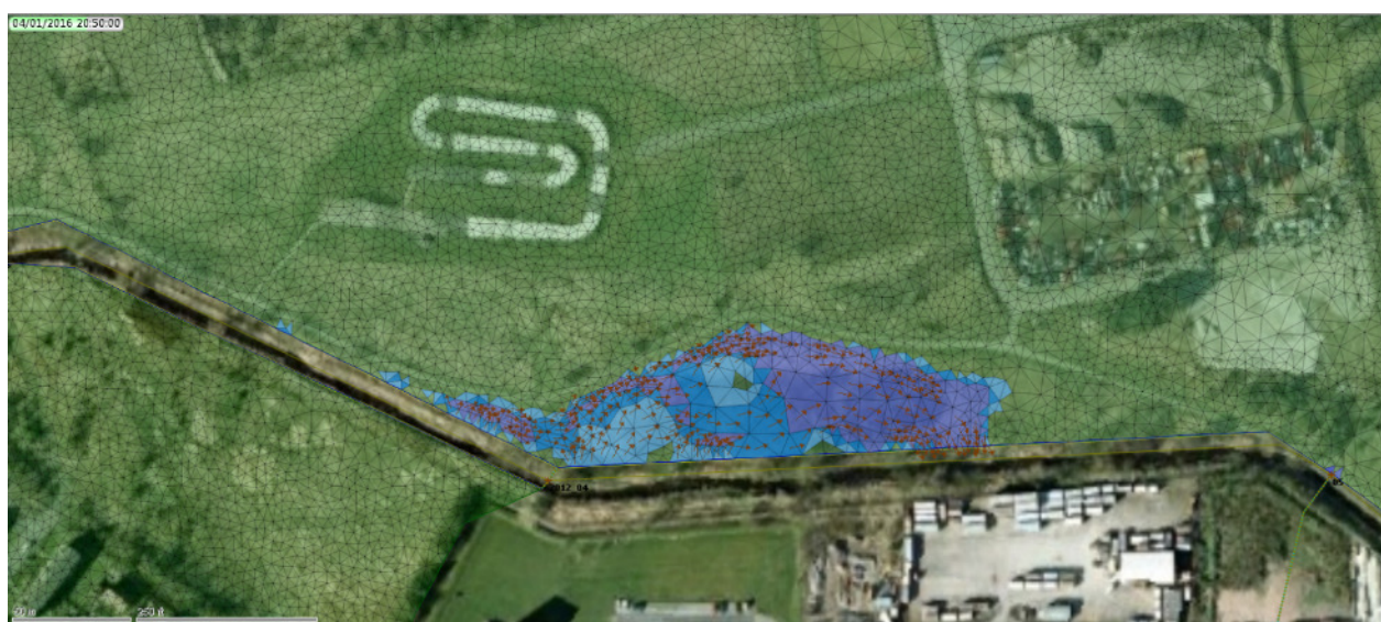
Figure 5a: Flow direction showing water leaving the channel at node 04, spreading towards the east, with some water going back into the river mid-way between 04 and 05.
