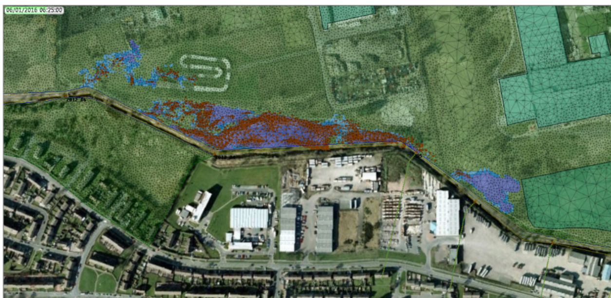
Figure 5d: Water moving across the BMX track
