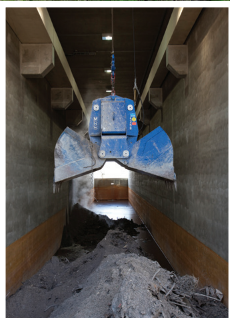
A typical bunker for bottom ash
