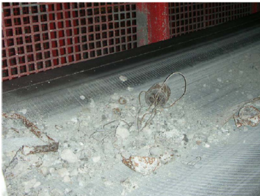
Plate 6.6 Typical IBA being conveyed to the bunker
