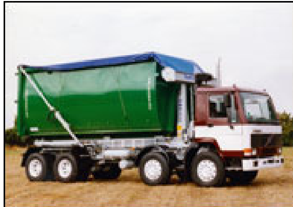
Photo of a typical Hookloader vehicle with a container mounted showing the automatic sheeting system
