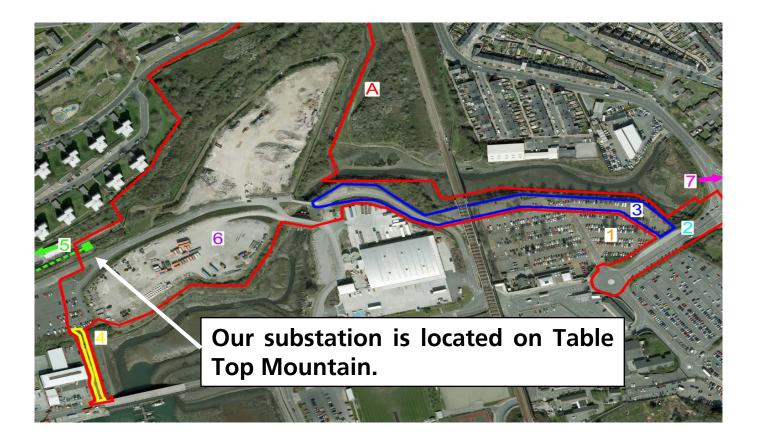
Power is delivered via an 11kV cable from the Bull Point substation
