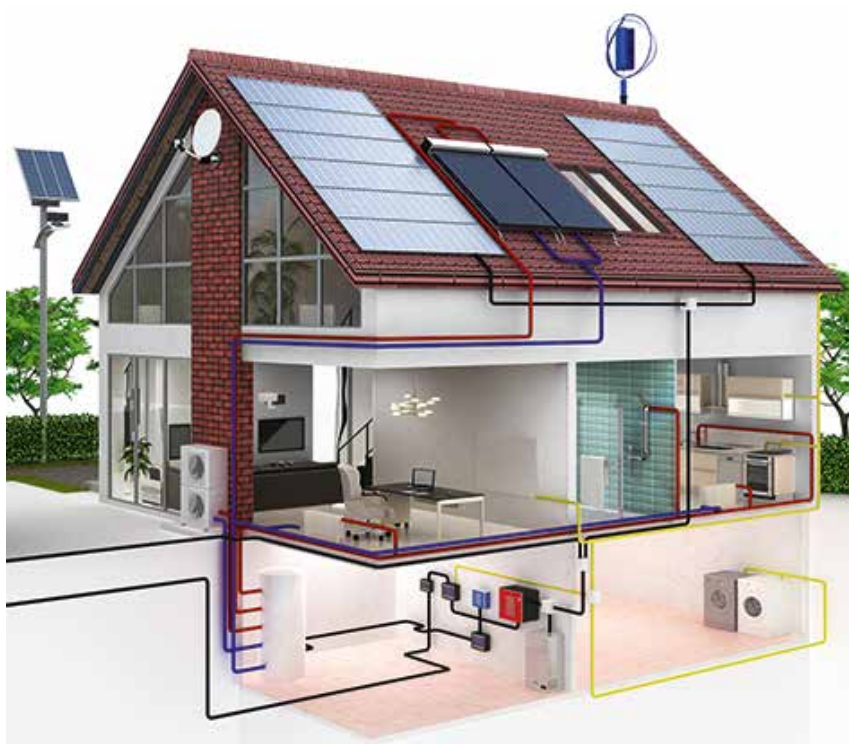
The solar thermal energy plant and heat pump supply the house with electricity and heat
