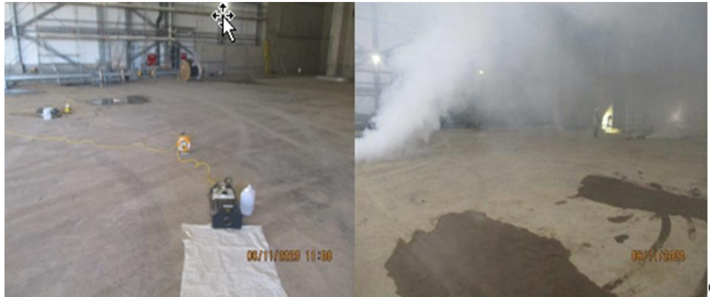
Smoke Test carried out in Tipping Hall
